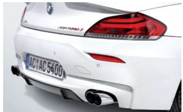
Acoustic and visual highlight: The AC Schnitzer sports exhaust system with stainless steel rear silencer and chromed tail pipe in Racing design.
