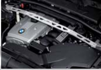
Full torsional rigidity: The AC Schnitzer aluminium strut brace
